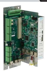
The **QE20-FP2000 Controller Module** is the 'brain' of the QE20 EWIS system.
